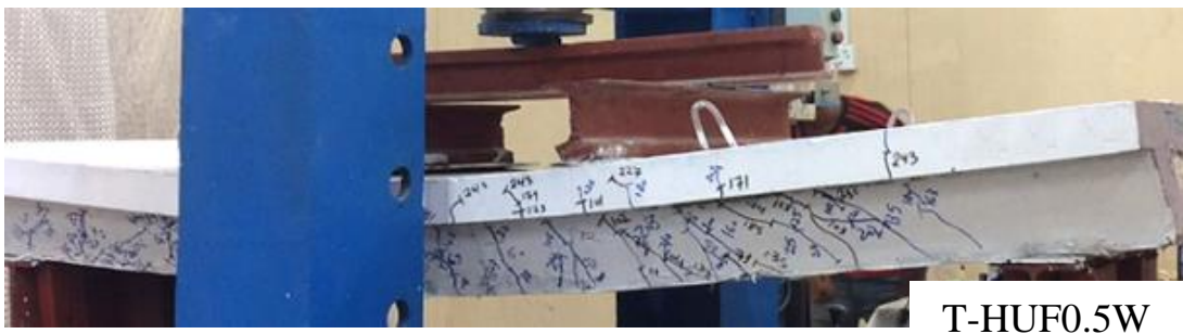
Figure (7): failure mode of specimen T-HUF0.5W.
