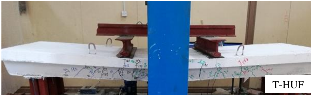
Figure (6): Failure mode of specimen T-HUF.
