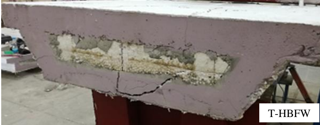
Figure (8): Failure mode of specimen T-HBFW.
