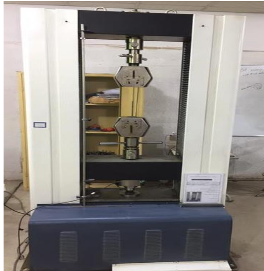
Figure (1): The instrument which is used for the yield stress
