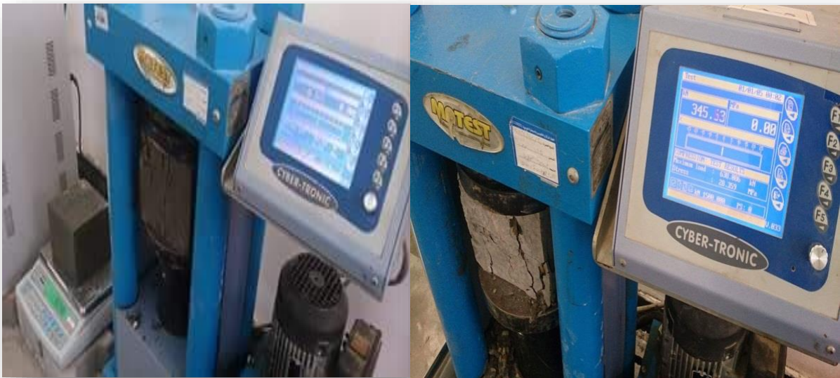
Figure.4 : Cube samples during compression test
