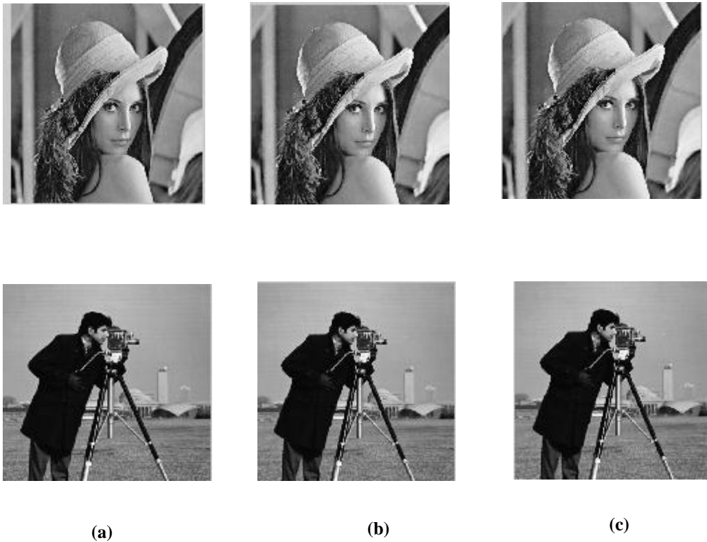
Figure (2) Results of applying traditional IBTC (a) Original image(b) Reconstructed image (c) Embedding image with payload (1024)
