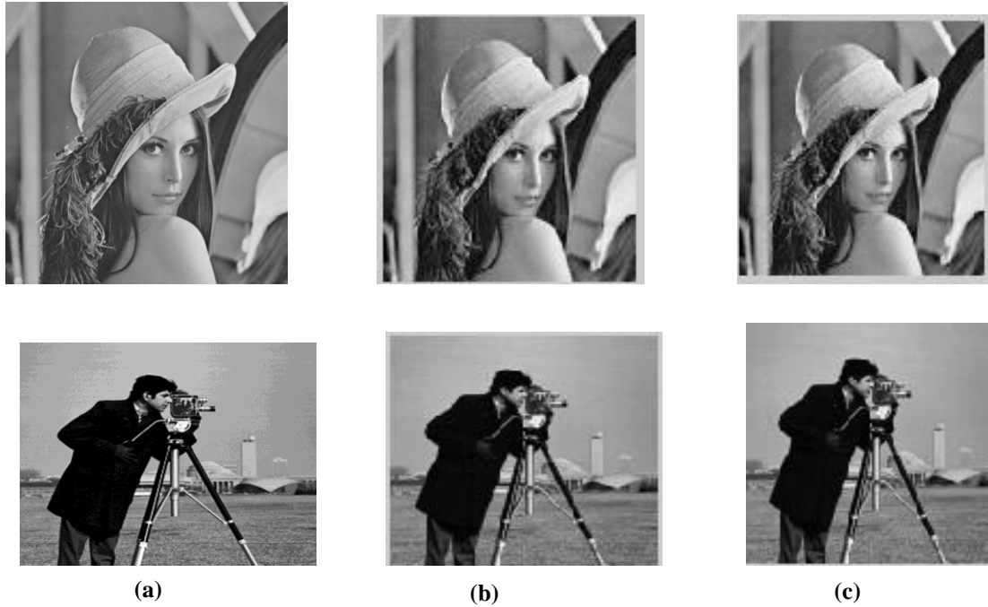
Figure (1) Results of applying traditional BTC (a) Original image(b) Reconstructed image (c) Embedding image with payload (1024)
