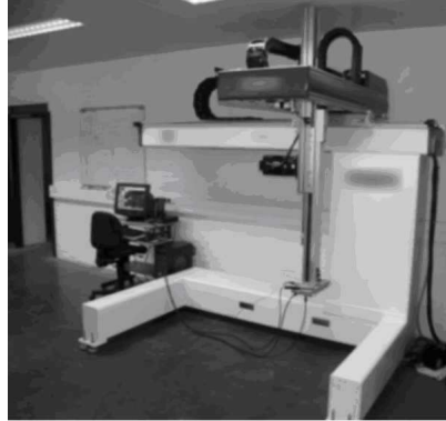
Figure 8: Overview of the first test-setup prototype (stroke [mm]: X-1000 Y-400 Z-800, max. feedrate: 120 \text{ m}\cdot\text{min}^{-1} , max. acceleration: 4 \text{ m}\cdot\text{s}^{-2} ).
