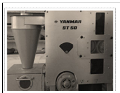
Fig 1 The machine t(type Yanmar) wich is used for hulling paddy
