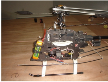
Figure 1: Implemented rotorcraft UAV.
