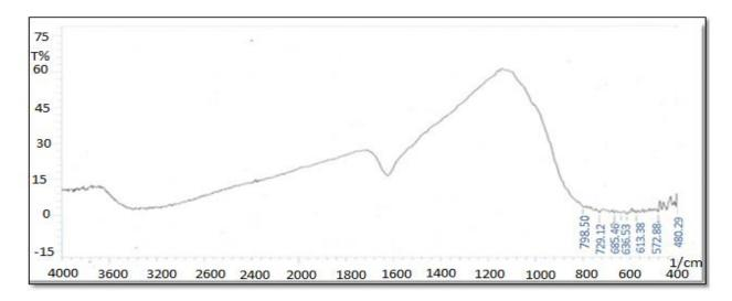
Figure (2). FTIR transmittance spectrum of TiO<sub>2</sub> annealing at 400°C for 120 min.
