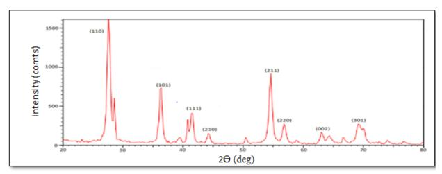
Figure (1). XRD patterns of TiO<sub>2</sub> annealing temperature at 400°C for 120 min.
