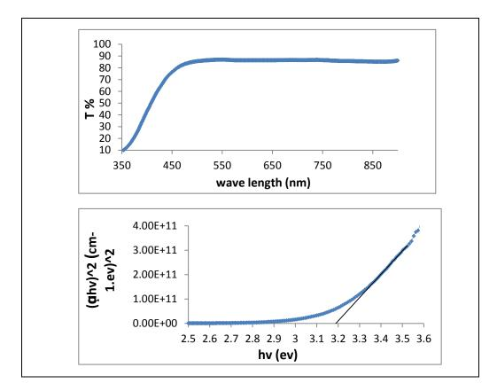
Figure (5). Optical Transmission as a function of wavelength for r-TiO<sub>2</sub> annealing at 400  $^{\circ}$ C for 120 min.
