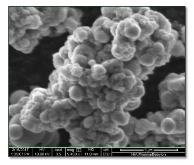
Figure (4). SEM image for TiO<sub>2</sub> nano powder at 400°C for 120 min.
