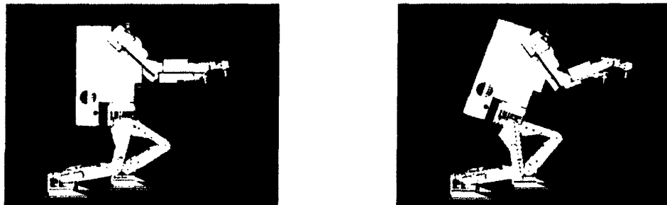
Fig. 5: The configurations of optimization (left: pre-optimized configuration, right: post-optimized configuration).
