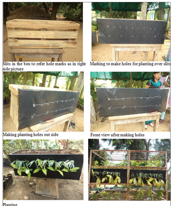
Plate 1: Fabrication of planter boxes for vertical garden system
