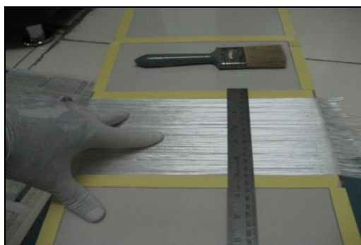
Fig 3. Fiber strands retained in parallel position and a series of molds are in line.
