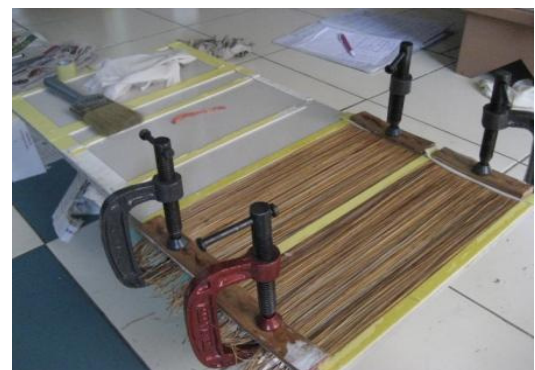
Fig 3. Dry fibers tend to curl and twist
