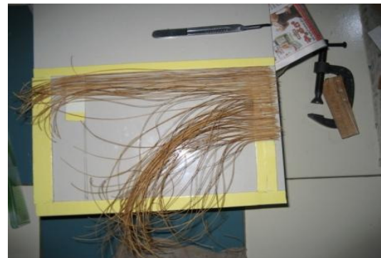
Fig 3. Dry fibers tend to curl and twist
