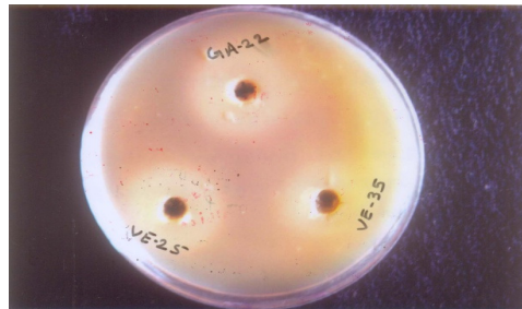
Plate 2. Actinomycetal isolate showing zone of inhibition against E. coli (agar well method antibiotic)
