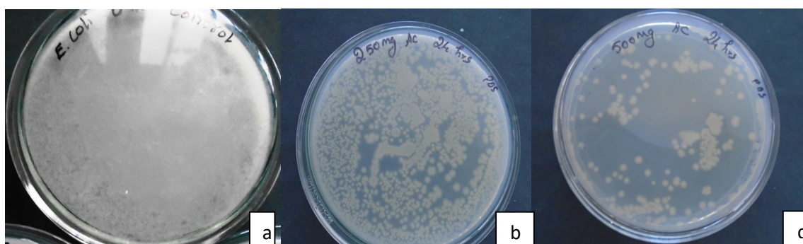
Fig. 4. Image showing colonial growth inhibition of E.coli after 24 hours incubation by shake flask test a.Control, b. Reduction in number of colonies after 24hours at 250mg of activated carbon, c. Reduction in number of colonies after 24hours at 500mg of activated carbon.
