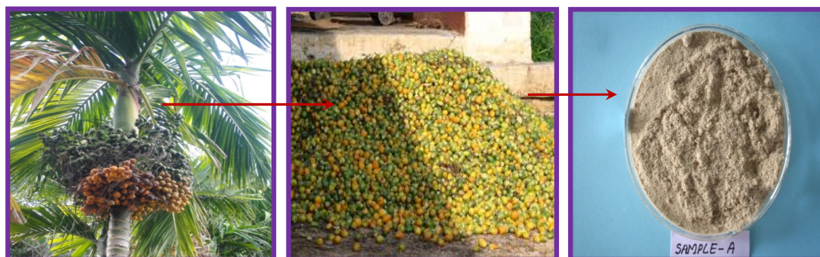
Figure 2: A. Areca nut palm (plant), B. Areca nut husk and C. Areca nut husk fine sized powder (0.28±0.01mm).
