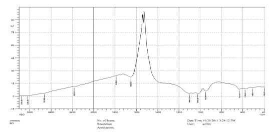
Figure 5 FTIR of extracted PHA sample
