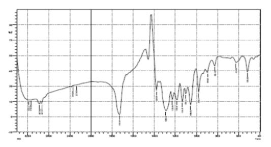
Figure 4 FTIR spectra of Standard Polyhydroxy-3-Butyric acid
