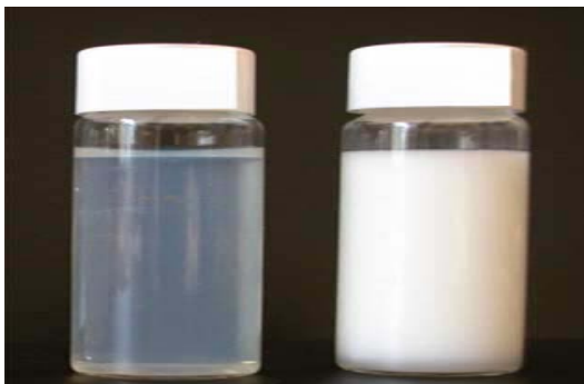
Fig.1. Nano-emulsion (left) with dia 35nm and a macro-emulsion (right) with dia 1 \mu m
