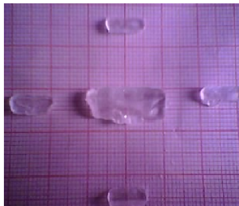
Fig 1. As-grown crystal of ZTTC
