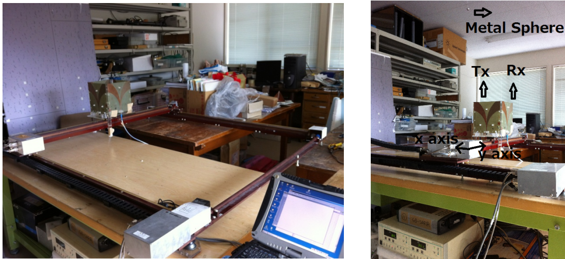
Fig. 3.4. Configuration of Experiment with xy positioner and Vivaldi antennas
