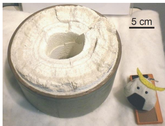
Figure 1-3 Silica scale of the Yamakawa geothermal plant, Kyusyu, Japan (displayed at the showroom of the Yamakawa geothermal plant, Japan).
