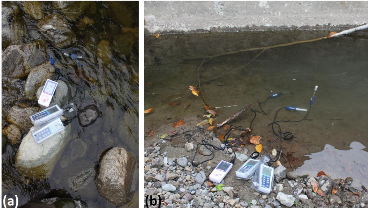
Figure 7.3 Measurement of chemical parameters at main stream (a) and dammed pool (b)
