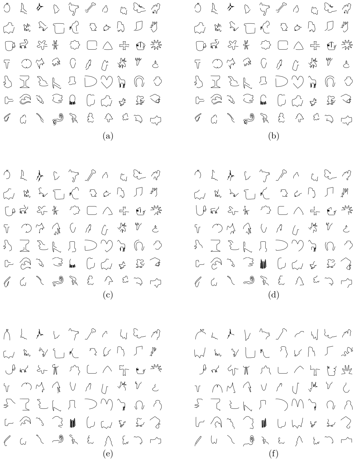
Fig. 4.8 Examples of open contours constructed with the MPEG-7 CE-Shape-1 part B data set shown in Fig. 4.7. The open contours are certain ratios (99%, 90%, 80%, 70%, 60%, 50%) of the length of the closed contours of the original shapes in the data set. Examples of open contours for the ratios of 99%, 90%, 80%, 70%, 60%, and 50% are shown in (a)-(f).
