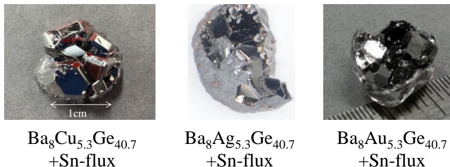
FIGURE 5.1: The grown single crystals of noble metal containing clathrates, BMG, where M = \text{Cu}, \text{Ag}, \text{Au} .
