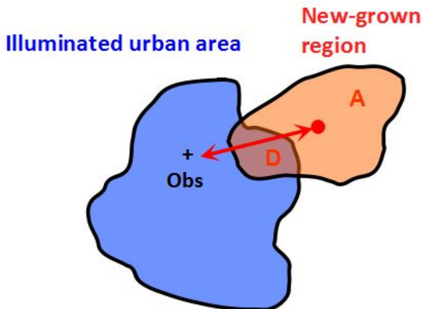
Figure 2.5 Schematic figure of the definitions of rapid urbanization area ( A ), distance ( D ). The cross mark (+) indicates the location of observation site. The blue area denotes illuminated urban area, which is usually used to stand for city size. The orange area indicates new-grown region defined by night light increase. The size of this area is the rapid urbanization area ( A ) used in our definition. The red dot is the mass center of rapid urbanization area, distance ( D ) is calculated as the distance between the mass center and observation site.
