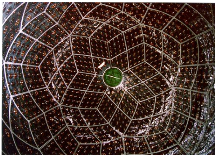
Fig 3.12: The picture of PMT geometry inside ID before LS filling. The spherical shape is formed with combination of the diamond shape structures holding 16 PMTs. The transparent acrylic walls cover each diamond shape structure to separate BOO and BOI.
