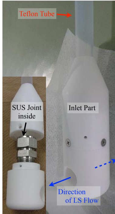
Fig 6.20: Picture of teflon tube and inlet part. The teflon tube is connected to inlet part with joint portion made of stainless steel (SUS). The directions of LS flow is horizontal not to make vertical convection in IB because the filling is operated by pile-up of LS layers.
