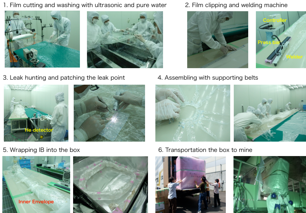
Fig 3.19: The pictorial procedure of inner balloon fabrication. The numbers above each picture correspond the numbers of steps in the procedure of the fabrication.
