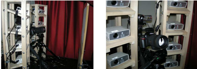
Fig. 10. Experimental system. Left: The layout of eight projectors and a screen. Right: A video camera (left) for the calibration and a still-image camera (right) for verifying the image quality of the realized images.
