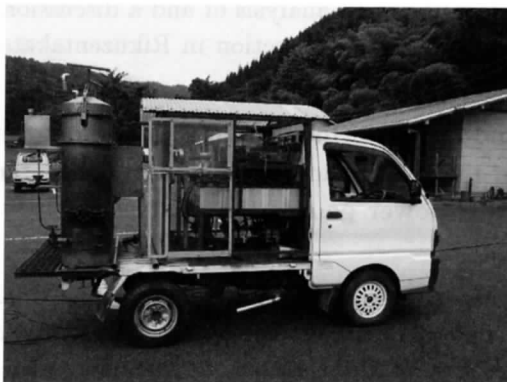
Plate. 4 Equipment of charcoal power generation
