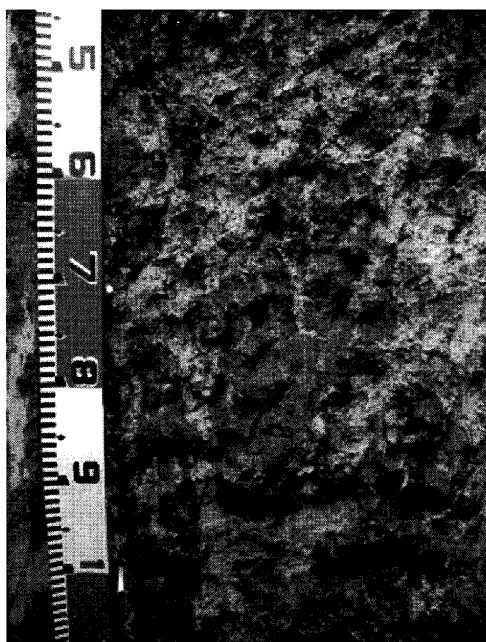
Fig. 6. Plinthites through the Btv horizons from a paddy soil profile (Plinthaquults) on Chungli terrace in northwestern Taiwan. The dark colored zones indicate Fe-rich masses and the light gray zones are redox depletions. The scale unit is 1 cm.
