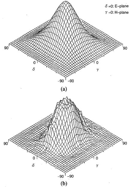
Fig. 10. The calculated and measured two-dimensional radiation patterns of a microstrip patch antenna on a dielectric hemisphere of 100 mm diameter ( $\epsilon_{r1} = \epsilon_{r2} = 2.13$ ). (a) Theory. (b) Experiment at 52 GHz. The scale is linear in power.
