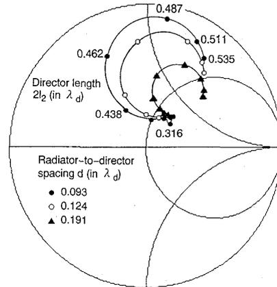
Fig. 3. The calculated input impedance of a Yagi-Uda antenna on a dielectric hemisphere ( $\epsilon_r = 2.13$ ).
