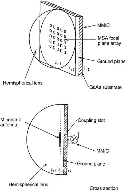
Fig. 8. The configuration of a two-dimensional microstrip patch antenna imaging array.
