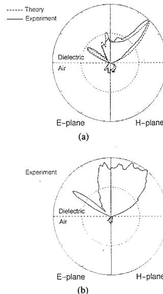
Fig. 7. The calculated and measured radiation patterns of a trap-loaded antenna on a dielectric hemisphere ( $\epsilon_r = 2.13$ ) of 100 mm diameter. (a) Dipole. (b) Yagi-Uda ( $2l_1 = 0.5\lambda_e$ ,  $2l_2 = 0.414\lambda_d$ ,  $d = 0.124\lambda_d$ ). The scale is linear in power; --- theory, — experiment at 50 GHz.
