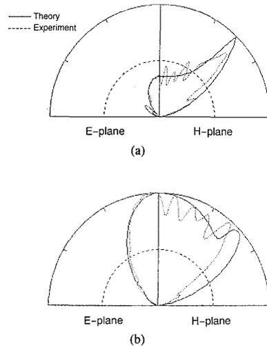
Fig. 2. The calculated and measured radiation patterns of an antenna on a dielectric hemisphere ( $\epsilon_r = 2.13$ ) of 100 mm diameter. (a) Dipole. (b) Yagi-Uda ( $2l_1 = 0.5\lambda_d$ ,  $2l_2 = 0.462\lambda_d$ ,  $d = 0.093\lambda_d$ ). The scale is linear in power; — theory, --- experiment at 50 GHz.
