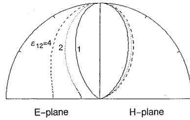
Fig. 9. The calculated radiation patterns of a microstrip patch antenna on a dielectric hemisphere for various  $\epsilon_{12}$ , where  $\epsilon_{12}$  is the ratio of the dielectric constant of the substrate ( $\epsilon_{r2}$ ) to the lens ( $\epsilon_{r1}$ ). The scale is linear in power.
