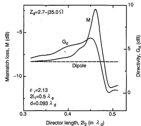
Fig. 4. The calculated directivity and mismatch loss of a Yagi-Uda antenna ( $2l_1 = 0.5\lambda_d$ ,  $d = 0.093\lambda_d$ ) versus director length  $2l_2$ . The diode impedance is  $2.7 - j35.0 \Omega$ .
