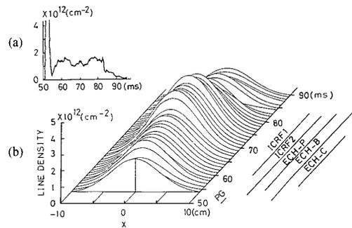
Fig. 12. The measurement of the time evolutions of the line-density (a) and line-density profile (b) at the plug cell in the Tsukuba GAMMA 10 plasma with a 10 element trap-loaded Yagi-Uda antenna imaging array at 70 GHz. The time sequence is as follows: following the gun-produced plasma injection (PG), the plasma is heated with ion cyclotron range of frequency (ICRF) powers and electron cyclotron heating (ECH) powers.
