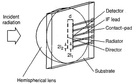
Fig. 1. Yagi-Uda antenna imaging array.
