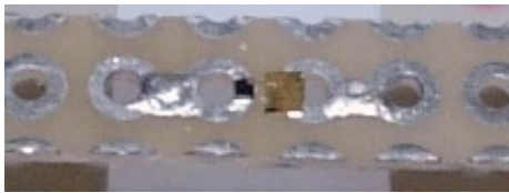
Figure 2. The diode chip mounted on FR-4 universal board.
