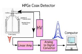
Figure 2. Electric diagram for the gamma ray measurement.
