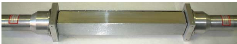
Figure 2. NaI(Tl) rod of 2 x 2 x 18 inch with Hamamatsu R1307 PMT.
