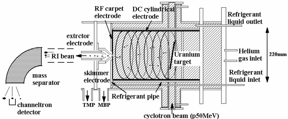
Figure 1. Schematic view of RFIGISOL2.
