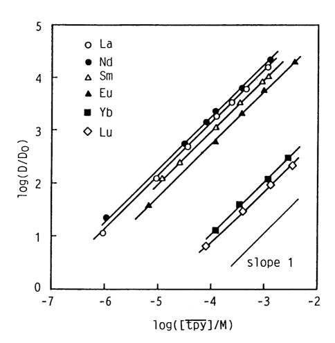
Fig. 2. Dependence of  $D/D_{\text{o}}$  on the equilibrium concentration of tpy in the benzene phase.
