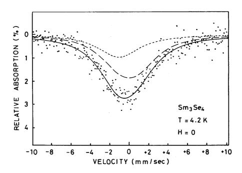
Fig. 1. Mössbauer spectra of  $\mathrm{Sm}_3\mathrm{Se}_4$  at 4.2 K. The lines are least squares fits to the data. Upper line is for  $\mathrm{Sm}^{2+}$ -ion, middle line is for  $\mathrm{Sm}^{3+}$ -ion and the lowest line is a total of them.
