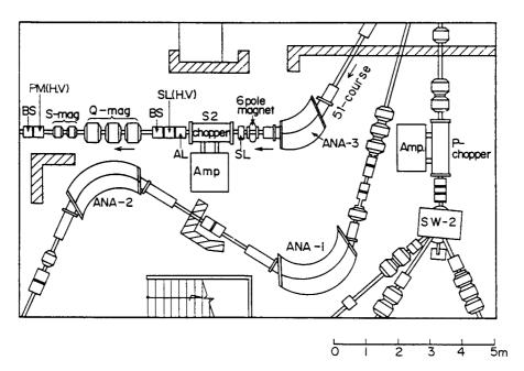
ANA: analyzer magnet, SL(H.V): slit(horizontal, vertical), SW: switching magnet, BS: beam stopper, S-mag: steering magnet, Q-mag: quadrupole magnet, AL: alumina monitor, PM: profile monitor. Arrows (+) show the direction of beams.
