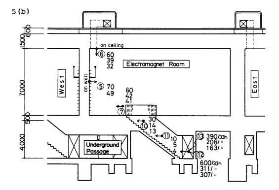
Fig. 5(a,b). Gamma-ray doses in mrem with 25 MeV deuterons. Figures from the upper line to the lower show those with film badges, TLDs (UD-200S), TLDs (UD-137N) respectively. -: not measured.
