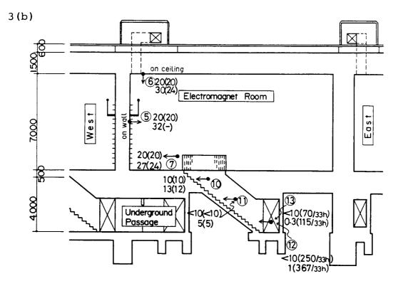
Fig. 3(a,b). Thermal neutron doses in mrem with 35 MeV protons and 25 MeV deuterons. The upper line figures show the data with Film-badges, and lower those with TLDs. Figures in parentheses show those on deuterons. -: not measured.
