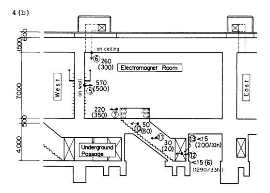
Fig. 4(a,b). Fast neutron doses in mrem with CR-39. Figures outside and in parentheses show the data obtained with 35 MeV protons and 25 MeV deuterons, respectively. Datum in square bracket was obtained with a rem counter. -: not measured.
