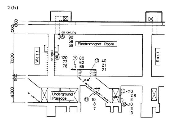
Fig. 2(a,b). Arrangement of detectors and γ-ray doses in mrem in the electromagnetic room (a: plane figure, b: cross sectional view) with 35 MeV protons. Circles (•) show the points measured and arrows (+) attached to the circles the directions of the detectors. Detectors were set at 1 m high except for Nos. 5 and 6. Figures from the upper line to the lower show those obtained with film badges, TLDs (UD-200S) and TLDs (UD-137N), respectively. -: not measured.
