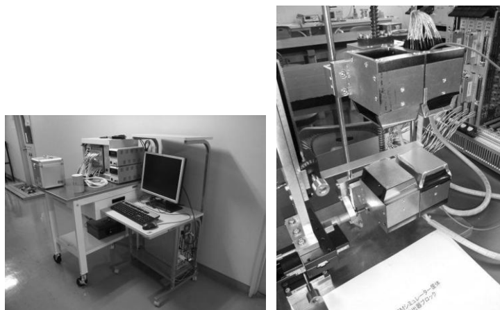
Figure 2. Left is the PEM simulator. The PEM simulator is a subset of the PEM scanner and used for the diagnosis of the crystals and the PMTs. Right is a close up of the detector units.
