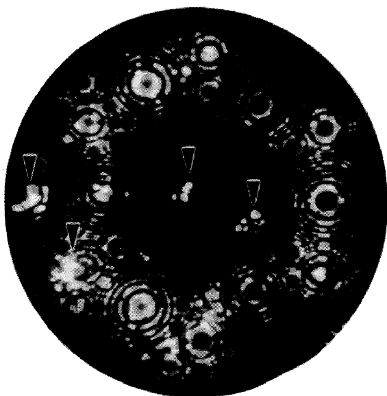
Fig. 1 He ion image of Al-6at.%Ag alloy aged at 130°C for 60 h.
