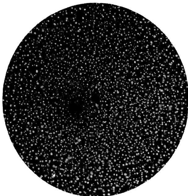
Fig. 11 Ne field ion micrograph of melt-spun \text{Fe}_{73.5}\text{Si}_{13.5}\text{B}_9\text{Nb}_3\text{Cu}_1 amorphous alloy.
