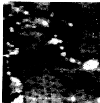
Fig. 1. Filled state image of the clean C-terminated 6H-SiC(0001) 2\sqrt{3} \times 2\sqrt{3} surface. Bias = -1.5 volts. Image size = 160Å x 160Å.
