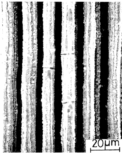
Figure 5 Appearance of Nb 3 Sn pre-stressed up to \sigma_{c,L} = 258\text{MPa} . The co-existence of the broken and unbroken Nb 3 Sn indicates that the strength of each Nb 3 Sn filament is different.
