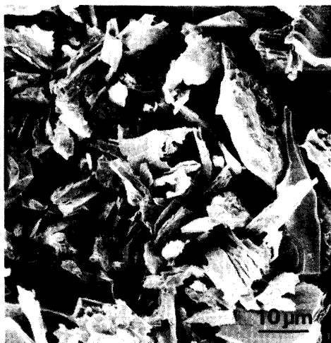
Fig. 6 Scanning electron micrographs showing the morphology of the ribbon sample at the initiate stage of oxidation for an amorphous Zr_{70}Au_{30} alloy aged for 2 days at R.T. in air with a relative humidity of 100 %. (b) is an enlarged micrograph taken from the region A in (a), and (c) and (d) present enlarged micrographs taken from the directions of the arrows B and C, respectively, marked in (a).
