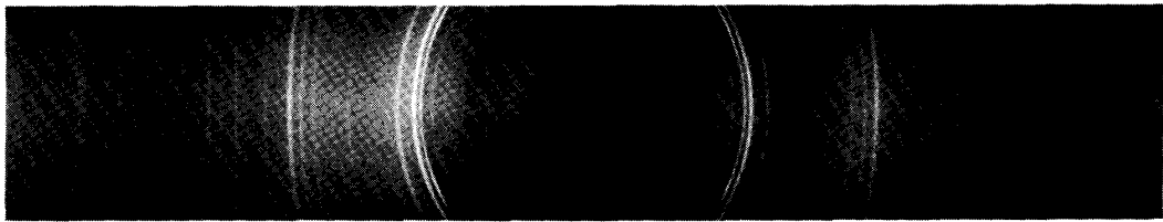
Fig. 3. X-ray diffraction pattern of Fe-17% B alloy annealed at 100 kbar and 460°C for 21 hours and quenched to the ambient conditions, showing the formation of the DO_e -type Fe_3B . Filtered FeK\alpha radiation.
