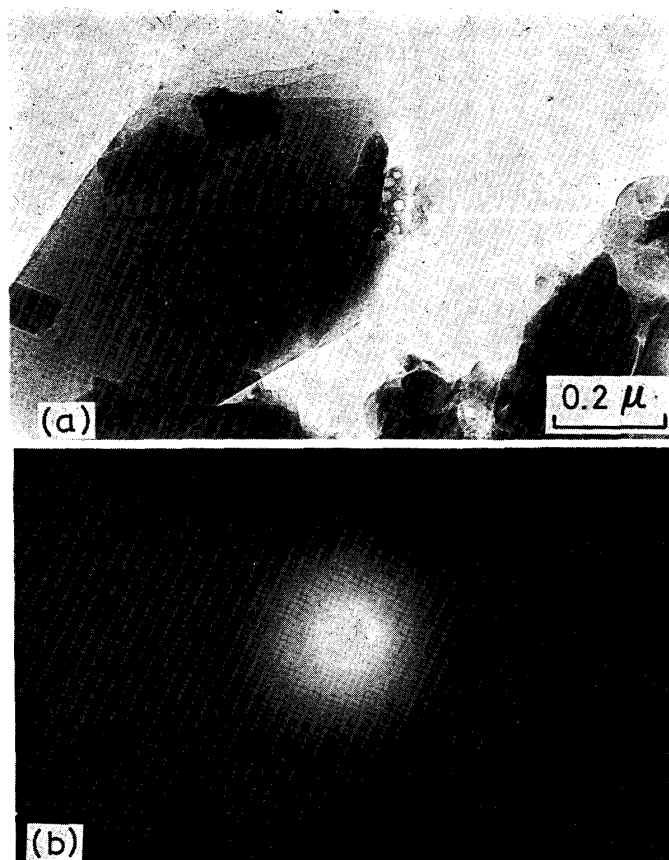
Fig. 3. Electron micrograph (a) and electron diffraction pattern (b) of the CVD-amorphous \text{Si}_3\text{N}_4 prepared at T_{\text{dep}}=1300^\circ\text{C} , P_{\text{tot}}=10 Torr and \text{FR}(\text{SiCl}_4)=170 \text{cm}^3/\text{min} .
