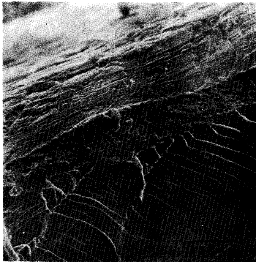
Photo. 3. Dimples of unirradiated Nb fractured at liquid N_2 temperature.
