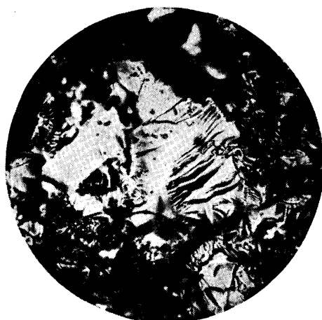
Photo. 1. Microstructure of a \{111\} surface of Ge crystal polished with #60 SiC powder. ( \times 270 )
