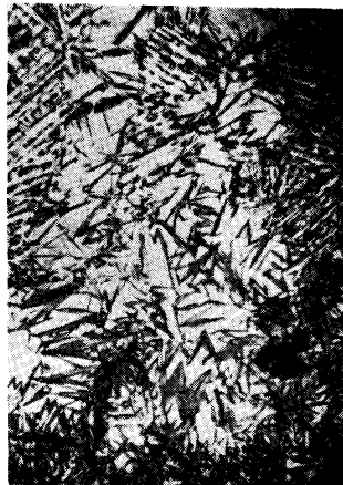
Photo. 4. Microphotograph of martensite in heat-affected zone.
