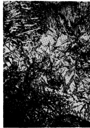
Photo. 3. Microphotograph of martensite in heat-affected zone.
