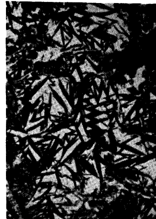
Photo. 6. Microphotograph of martensite in heat-affected zone.
