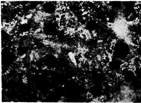
Photo. 3. Pearlitic type of nodular graphite cast steel.
