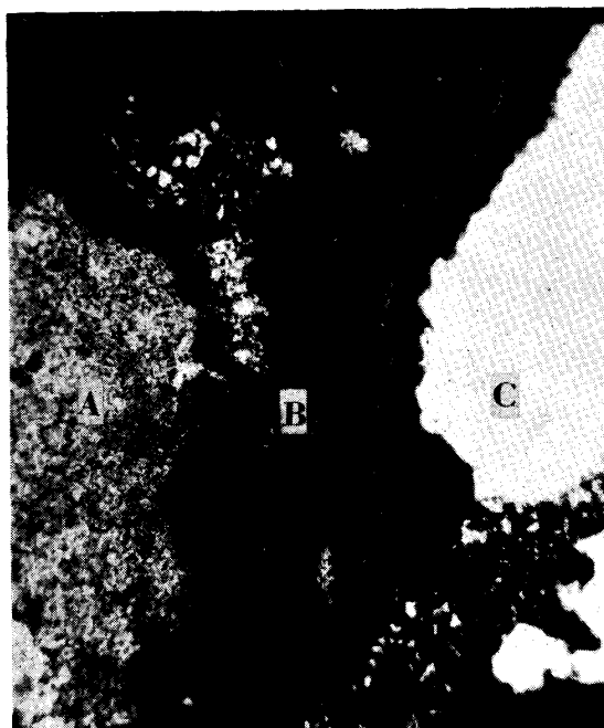
Photo. 1. Photomicrogram of oxidized siderite from Fukuô Mine. (Thin section, open nicol, \times 50 ) A : Siderite B : Goethite C : Cavity
