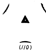
Fig. 5. \{111\} light figure of 40% Cu alloy crystals etched with boiling sat. aq. sol. of \text{FeCl}_3 \cdot 6\text{H}_2\text{O} for 3.5 min.
