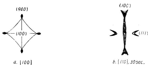
Fig. 7. \{100\} and \{110\} light figures of 90%Cu alloy crystals etched with boiling sat. aq. sol. of \text{FeCl}_3 \cdot 6\text{H}_2\text{O} for 30 sec.
