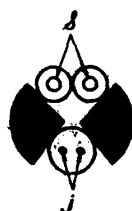
Fig. 3. Sectional view of the bundle binding the specimen, thermojunction and their holders.
